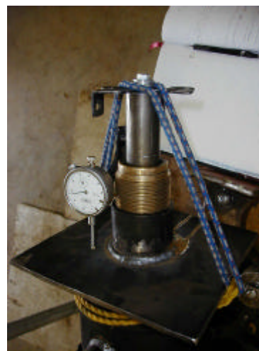
Figure 4. Details of expansion measurement.
